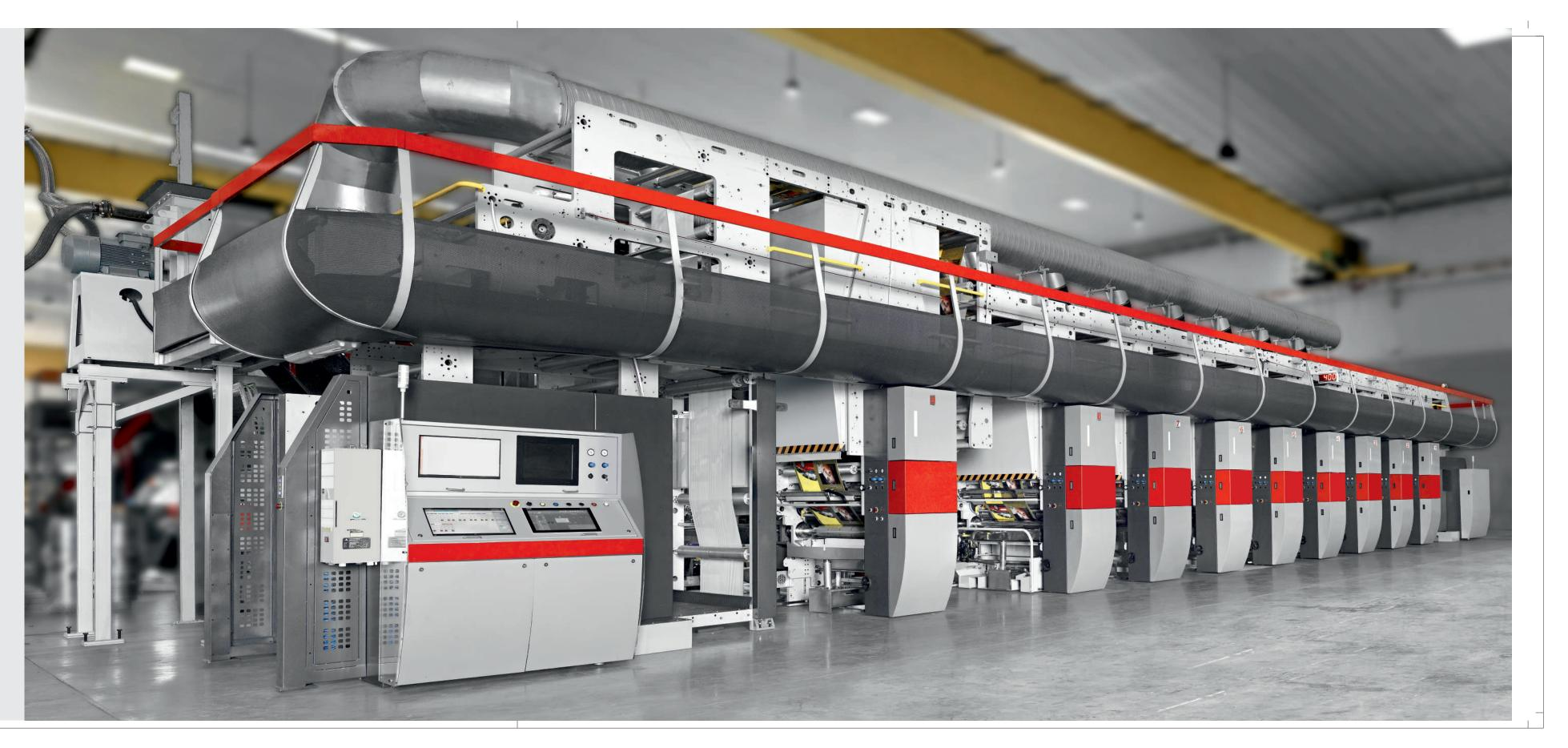
450 MPM ROTOGRAVURE PRINTING PRESS WITH SHAFTED OR SHAFTLESS CYLINDER CHUCKING
